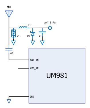
Figure 3-2 UM981 External Antenna Feed Reference Circuit
