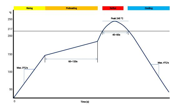
Figure 4-1 Soldering Temperature (Lead-free)
