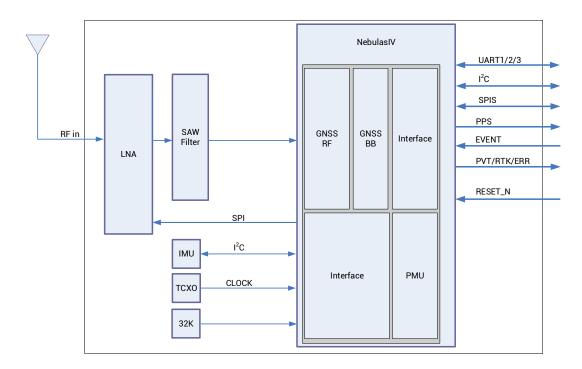
Figure 1-2 UM981 Block Diagram
