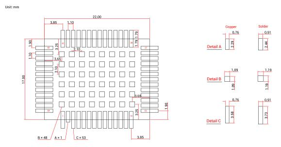
Figure 3-4 Recommended PCB Package Design
