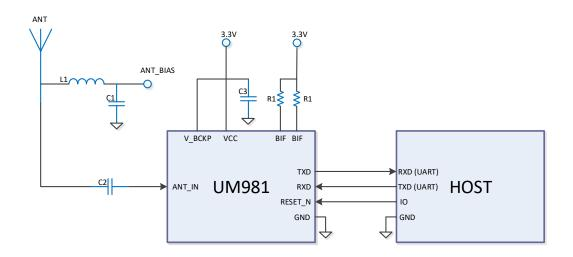
Figure 3-1 Recommended Minimal Design
